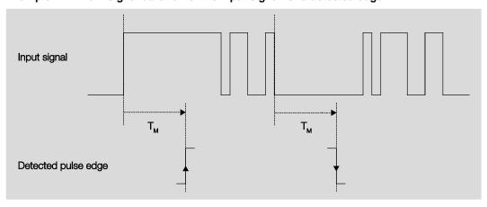
In only two cases, no further edge changes occur within the minimum signal duration  $T_M$  after a change of edge. For this reason, only both of these are detected as valid.
