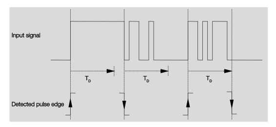
After detection of an edge on the input, further edges are ignored for the debounce time T<sub>D</sub>.
