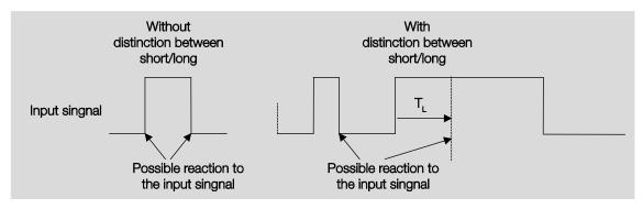
$T_L$  is the time duration from where a long operation is detected.
