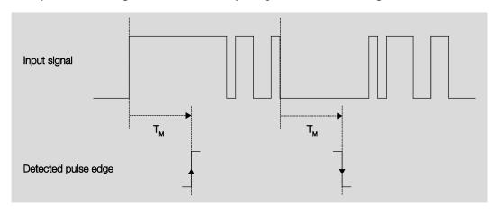
In only two cases, no further edge changes occur within the minimum signal duration T<sub>M</sub> after a change of edge. For this reason, only both of these are detected as valid.
