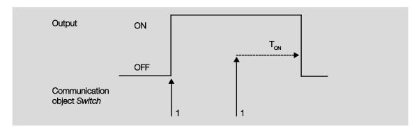
The response is the fundamental response of the staircase lighting function.
