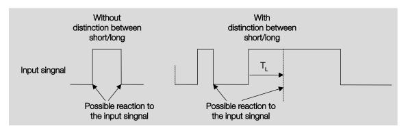
$T_L$  is the time duration from where a long operation is detected.
