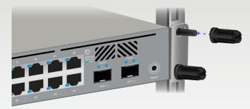
The S8-PoE switch has padding for desktop placement and notches for mounting on the included wall-mount bracket.
